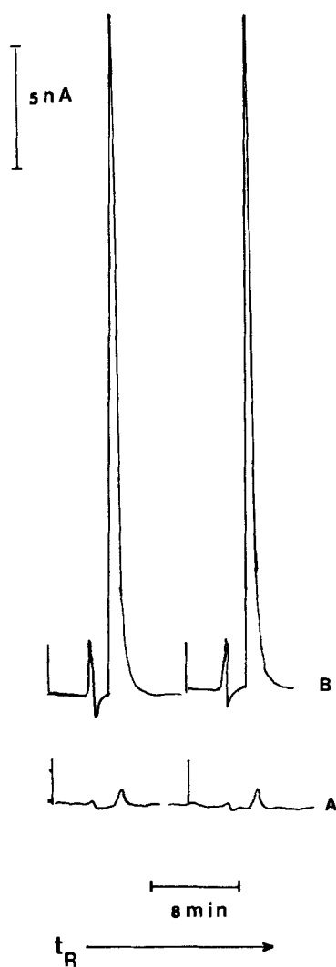
FIGURE 1. Chromatograms obtained at +0.30 V vs. Ag/AgCl for repeated injection of 30 ppm solution of NADH at (A) untreated and (B) electrochemically pretreated glassy carbon electrodes. Injection volume: 20 \mu l; flow rate: 2.0 ml/min.
